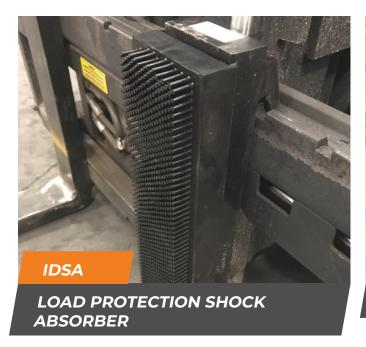
The load protection shock absorber has been designed to reduce damage to fragile loads from the fork back height when being loaded or unloaded via a forklift truck. This helps eliminate the time and money lost decanting damaged stock. The load buffer simply attaches to the face of the fork and is held in place magnetically. Best suited to applications where the load face is uneven, such as glass bottles, the IDSA rubber fingers mould to the product giving increased protection.
