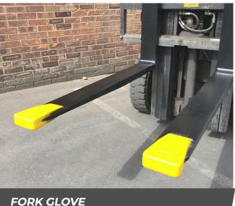
Specifically designed to greatly reduce product, pallet, and racking damage, while enhancing safety without affecting the operation effectiveness of the truck. The fork glove attaches to the tips of the forks by a specific bonding and must be applied to a new and undamaged fork surface.
