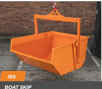
Our Boat Skips includes a specific self-dumping system, used for general muck and waste removal. These high-quality skips perform efficiently and safely as they are lifted and empty automatically without the need of any assistance. This feature eliminates the risk of danger to the personnel or operative alike. Robust manufacture to suit the condition and environment in which the skips work.
