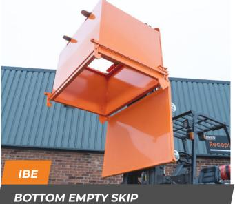
Automatic Bottom Empty Skips allow the simple but effective disposal of light to medium weight waste when being automatically emptied into high sided yard skips via the base release mechanism, without the driver leaving the safety of their seat.
