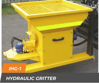
A hydraulically driven salt spreader/gritter, with safe and convenient fork pockets for front mounting. It is driven from the forklift truck's third service valve or side shift valve. Fitted with stainless steel double auger system which can spread all types of salt, with a 0.20m³ hopper to take around 250kg of salt.
